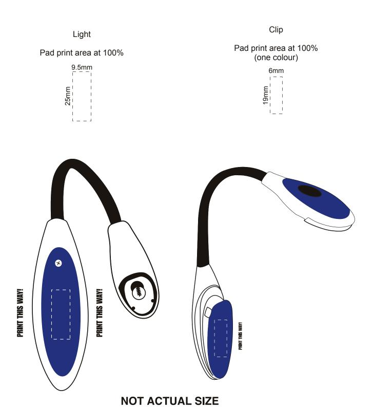
Clip Light Pad print area at 100% (one colour) Pad print area at 100% 9.5mm 6mm \* **PRINT THIS WAY! PRINT THIS WAY!** PRINT THIS WAY!
